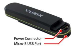
• Connect the USB Charge Cable to a USB power source providing a minimum of 1.5A. Most standard mobile phone chargers will be sufficient, however please refer to the annotations on your charger to ensure it will supply sufficient current.
